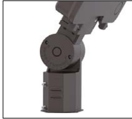
Slipfitter Mount An optional cast aluminum mast arm adapter secures fixture head to nominal 2-3/8" O.D. horizontal steel tenon arm.
