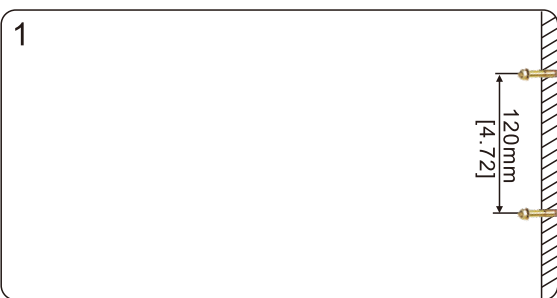
1. Drill 2x Ø10 hole for expanded screws, and fix them to the wall. (Horizontal distance: 171mm)
